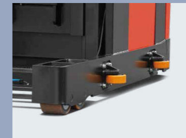
Rail guidance rollers (Opt.) can be fitted to the truck for VNA working
